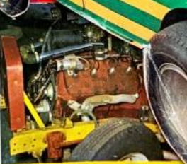
A flathead V8 Ford mill no less sits forward of the 1/8 in. firewall. Rad is from a Minor 1000!
