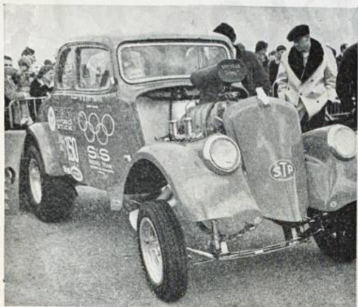
PACKED WITH POWER. —The 7½-litre Chrysler V8 engine, with G.M.C. supercharger, can be seen protruding from the engine room of Ken Pittman's drag coupe built around a 1933 Willys coupe. In spite of a "built-in headwing" it turned 10.52 sec. and went through the traps at 144 m.p.h.
