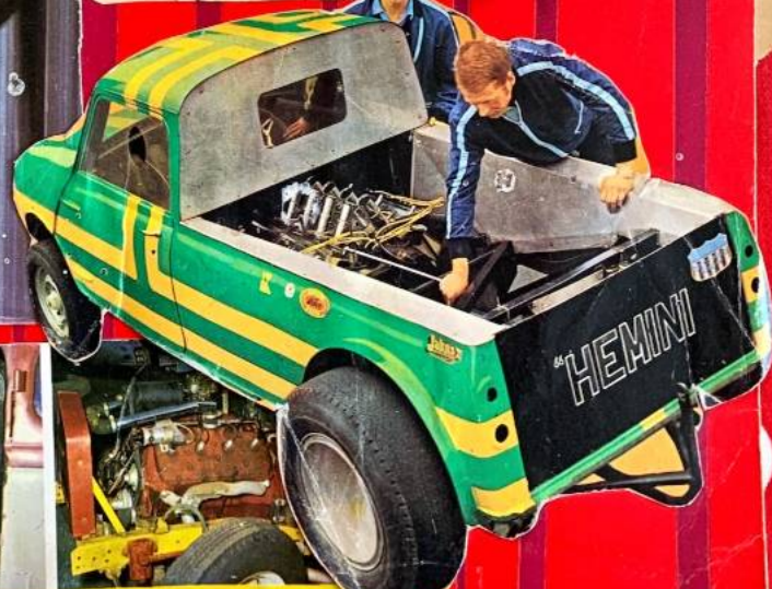
A flathead V8 Ford mill no less sits forward of the 1/8 in. firewall. Rad is from a Minor 1000!
