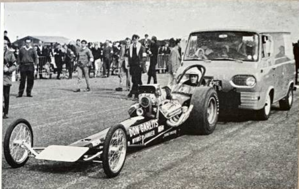
PUSH-START. —With a single high gear dragsters need to be doing about 20 m.p.h. before the engine can be started, and the system is to push them from the rear; Don Garlits is about to be started. Note the wind-deflector on the front axle.
