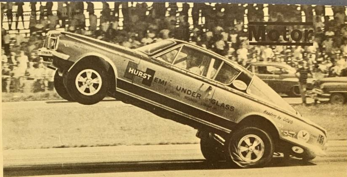
Wild Bill Shrewsbury in action with his Plymouth, which is rear engine! Small castors at the rear keep the body intact while the tyres do incredible things.
