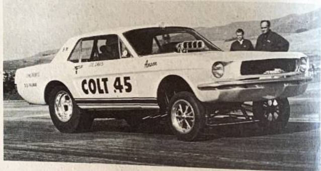
Below: The Mustang body on this car is a glass-fibre replica and the engine a Chevy V-8. The front suspension is minimal.
