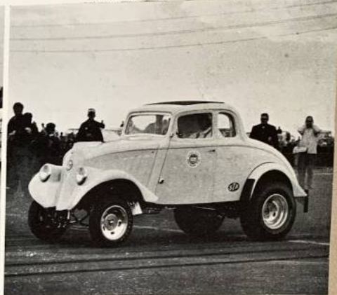
NO JOKE. —The incredible supercharged Chevrolet 6-litre V8-powered coupe of George Montgomery that made a best time of 10.37 sec. The finish of this car suggested "show, not go," but the performance was equally impressive.
