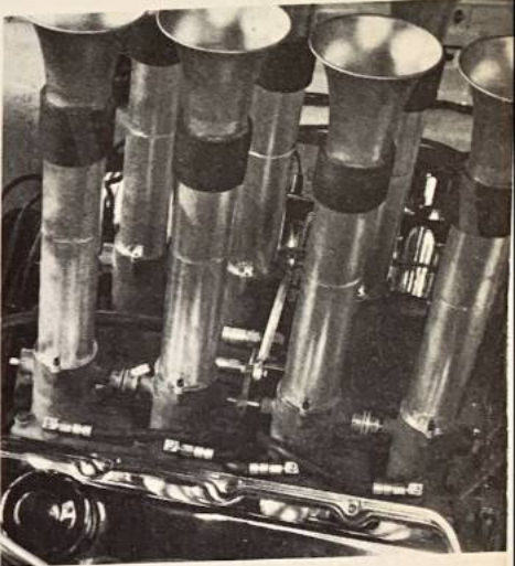
Stacks to suit all furnaces. Those at the top are used with manual gearboxes while the longer ones go on automatic transmission cars.
