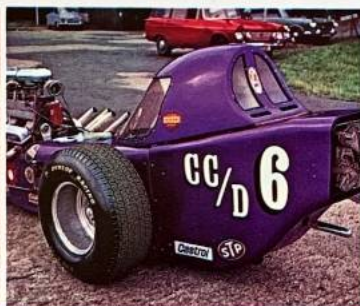
Driver is completely enclosed when the hood drops down — yet another safety factor. Note tail styling and neat drag chute locker. Bar is for push-starts.
