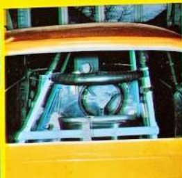
Interior has strong roll-cage in the event of a wipe-out. Rev and oil are only gauges
