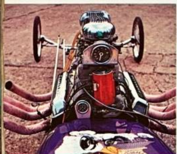
Driver should have no excuse for misreading that tach stuck up there on the Chevy mill. Note air scoop/ram for ensuring the carbs get maximum air.
