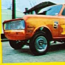
Front has been raised by lowering the spring perch—trims are 100E modded centres
