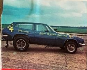
Side view of Whistler shows engine just too far forward to be a wheelie-machine. The castors are to prevent flipping
