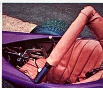
Everything in the driver's compartment is safety-angled, padded cockpit, bulkhead firewall, padded rollover bar, full-harness belts, and special wheel.
