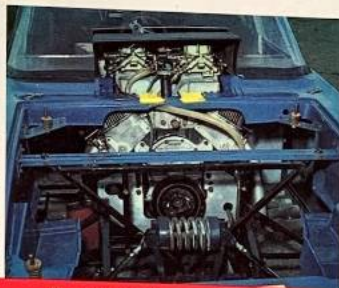
Seven-litre Chevy engine sits in the middle of the car. Pair of 4-barrel Holley carbs sits atop, well up in the air stream
