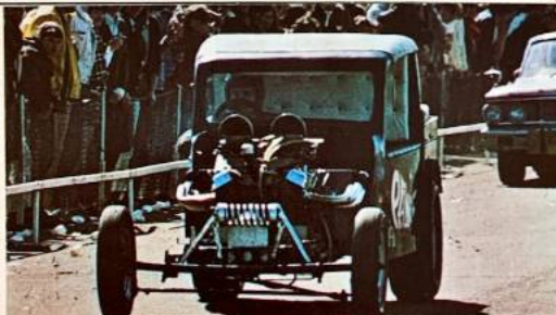
Dave Page's Panic is the ex-Stratton Hustler BSA pick-up—with a 5.3 Chevrolet slotted in, even BSA wouldn't know it
