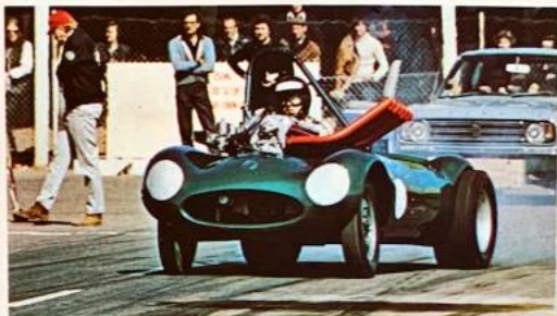
Colourful and deadly—that's John Williamson's Poison Ivy putting 3800 cc of Jaguar onto the road. Body is ex-Falcon
