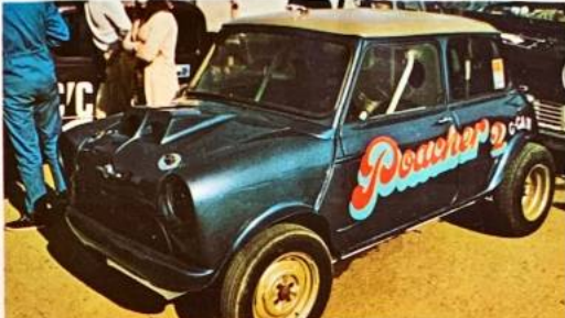
Most Mini—believe it or not is Defek Chester's Poacher. Like it's rear-wheel-drive—and like there's a 3.8 Jag mill
