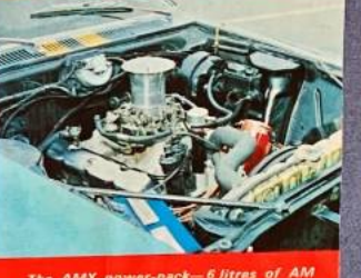
The AMX power-pack—6 litres of AM engine with a host of US drag goodies
