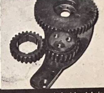
Chrysler camshaft drive (chain) is thrown away and replaced by a precision gear set that ensures spot on cam timing and eliminates chance of chain stretch
