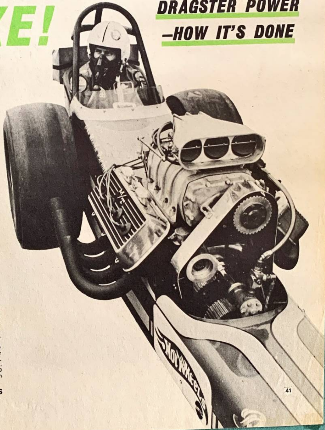
. . . sit in roller lifters on the wide lobe Engle camshaft. The lifters are paired and made from magnesium with steel rollers. With this set up friction is cut
