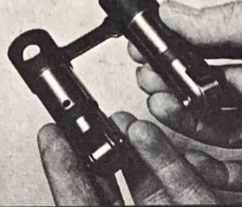
. . . sit in roller lifters on the wide lobe Engle camshaft. The lifters are paired and made from magnesium with steel rollers. With this set up friction is cut
