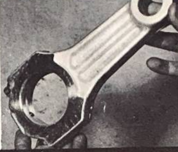
Forged aluminium connecting rods by Mickey Thompson—light and beefy. Note the pin for locating the bearing and the zig-zag join of the big end halves
