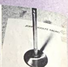
Valves are big — so big. This is fully shaped inlet (mark on paper are in inches) made in the US by Donovan Valves. Head porting is fully gas flowed
