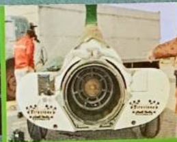
Business end of the Monster shows jet and after-burners, chutes and fluid suspension
