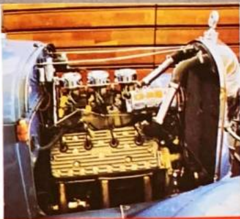
Swedish visitor—'49 Ford 5 window Coupe with 1949 flathead V8 power unit
