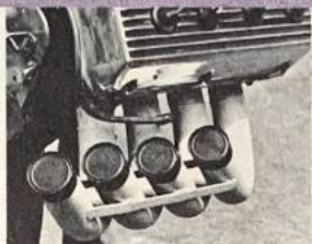
Heads are fully modified with Mickey Thompson rocker covers. Exhaust pipes, Zoomie Headers, and pipe into No 3 is for excess coolant blown off from block
