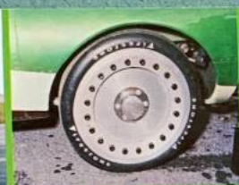
The Firestone-developed aluminium 22 in wheel is fitted with 300 psi 7 in wide slicks
