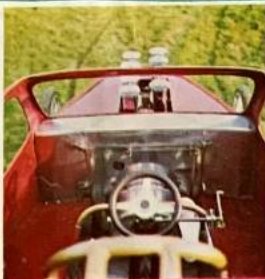
Driver's view includes a tach and little else in the way of instruments. Firewall is polished alloy and everything is aimed towards safety—rollbars etc
