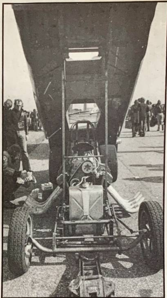
Chassis: Built of 1½in seamless tubing; wheelbase 117in Body: Built and painted by Barnet Motor Company Engine: 354cu in Dodge Hemi; forged steel crank; Isky 550 Magnum cam; Kieth Black budget head; Moon GMC blower; slider clutch from Scott Performance Industries; Lenco reverser unit; narrowed Olds' rear end; Wheels: Rear either with 10x15 Woolferace and M&H slicks ; front 15in American mags with Firestone racing tyres
