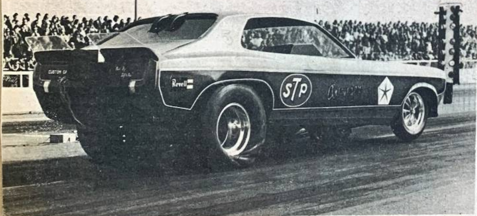
BLASTING off the line at the Santa Pod Raceway, Dennis Priddle's 'Avenger' lifts at front wheel and twists a rear tyre almost beyond belief. Starting with a low pressure, the tyre will 'inflate itself' be centrifugal force and heat build-up until it reaches full pressure for the rest of the run.
