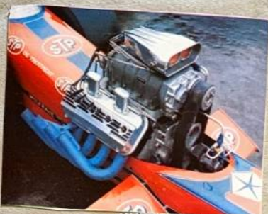
centre: the massive Chrysler-supercharged engine that gives driver Dennis Priddle about 1500 bhp to use
